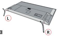
Place the TV set on a flat and clean surface with the panel facing downwards to avoid
